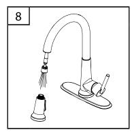
Turn on hot and cold water supplies. Pull the hose assembly out of the spout and remove the spray head by unscrewing it from the hose counter-clockwise. Be sure to hold the end of the hose down into the sink and turn the faucet on to the warm positions where it mixes hot and cold water. Flush water lines for one minute. Check for leaks. Re-tighten any connections if necessary, but do not overtighten. Re-install spray head by hand tightening it back onto the spray hose.
