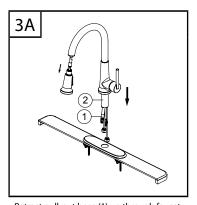
Retract pull-out hose (1) up through faucet body until the pull-out hose fitting is flush with the bottom of shank (2). Do not pull hose fitting past the shank. Insert faucet body through the hole in escutcheon.
