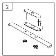
**Optional escutcheon installation**Install escutcheon over the three holes in the sink. From underneath sink, hand tighten mounting nut. Do not overtighten. Proceed to sten 3A
