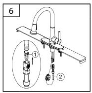
Align block (1) and tabs on quick connect. Push quick connect housing firmly upward and snap onto receiving block. Pull down moderately to ensure connection has been made. If it is necessary to remove quick connect, squeeze tabs on hose between index finger and thumb, then pull down to disconnect. After connecting the hose, install the weights at the lowest point of the hose (2).
