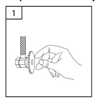
Locate water supply inlet and shut off water supply valve. These are usually found under the sink or near the water heater. Remove old faucet. Clean and dry sink surface area where new faucet will be mounted.
