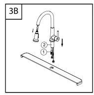
**Optional flange installation**Retract pull-out hose (1) up through faucet body, until the pull-out hose fitting is flush with the bottom of shank (2). Do not pull hose fitting past the shank. Insert faucet body through the hole.
