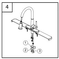
Install rubber washer (1), metal washer (2) onto the threaded mounting shank. Thread nut (3) onto mounting shank. Do not overtighten.
