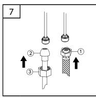
Make connections to water lines. Use 1/2" IPS faucet connections (1) or use supplied coupling nuts (3) with 3/8" OD ball-nose riser (2). Do not overtighten.
