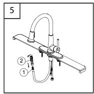
Screw quick connector (2) to the free end of pull-out hose (1).
