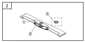
Place base plate (#2) and escutcheon (#1) on the sink. If you have no use for the escutcheon, please use seat (#3) to replace escutcheon and base plate.
