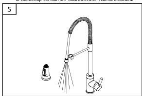
Turn on hot and cold water supplies. Remove the spray head. Be sure to hold the end of the hose down into the sink and turn faucet handle to the mixed position. Flush water lines for one minute. Check for leaks. Re-tighten if necessary, but do not overtighten. Attach the spray head to the hose
