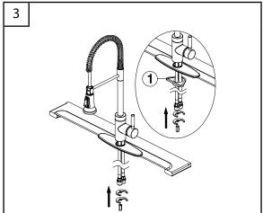
Insert supply hose assembly and thread rod through hole in sink (through center hole of escutcheon if used). Install rubber washer, metal washer and retaining nut onto the threaded rod. Firmly tighten retaining nut. Do not overtighten.
