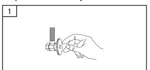
Locate water supply inlet and shut off water supply valve. These are usually found under the sink or near the water heater. Remove old faucet. Clean and dry sink surface area where new faucet will be mounted.
