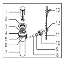
Drain Assembly Installation
